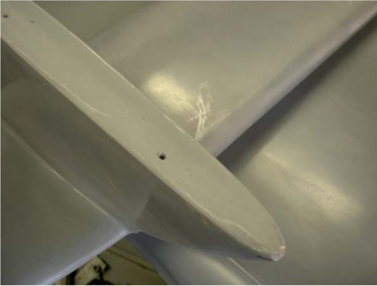
The vertical struts for the rear wing are drilled with pilot holes – in our case, we came in approximately 3” from each end, or approximately 5 ¼” between the centers.
