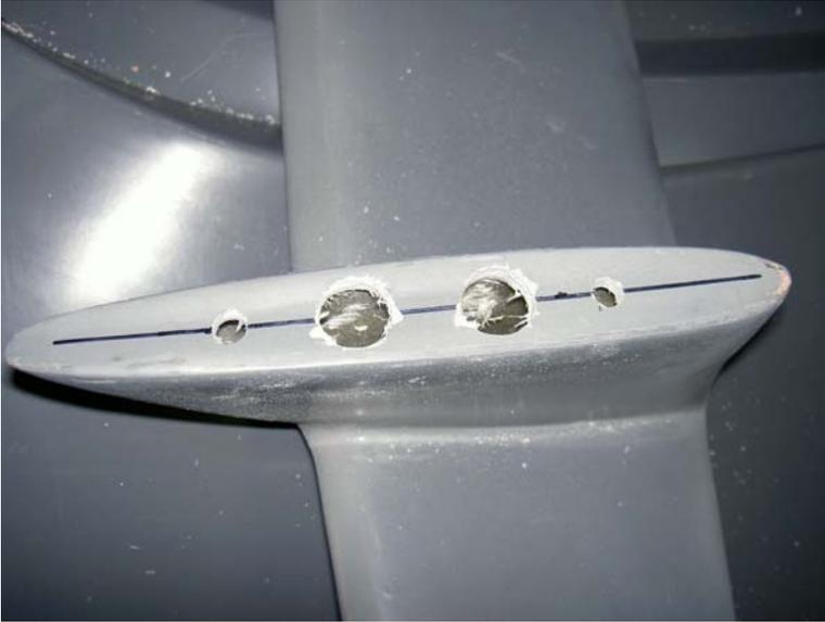
The pilot holes are drilled out to the 7/16" hole-size as suggested for the 3/8" T-Nuts we are using. We also add two 1" holes between the mounting holes. These will be used to insert the T-nuts from inside the wing vertical struts.
