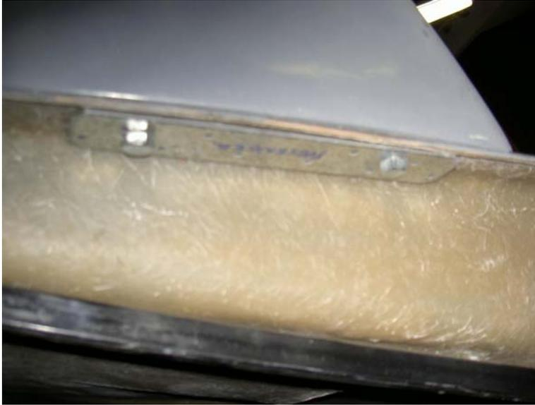
Tightening down the bolts, we have the wing installed properly.
