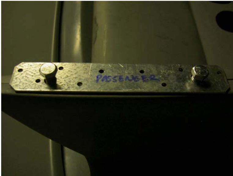
Once all the plates, struts, and holes have been checked for alignment and proper ease of installing, the rear wing is bolted to the rear hatch with the metal strips on each side below the rear engine hatch. The 3/8" bolts should have a lock washer on them to maintain security.
