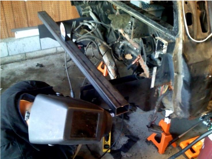
Rear of chassis/frame has been cut and removed.
