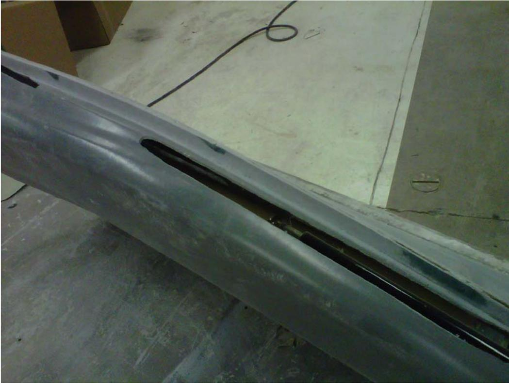
Door halves together with window slot
