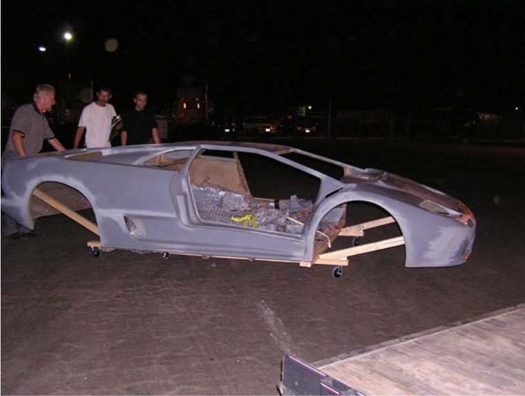
Body kit rolls easily on the body pallet with casters. Doors, hatches, and interior panels are tied inside of body kit.
