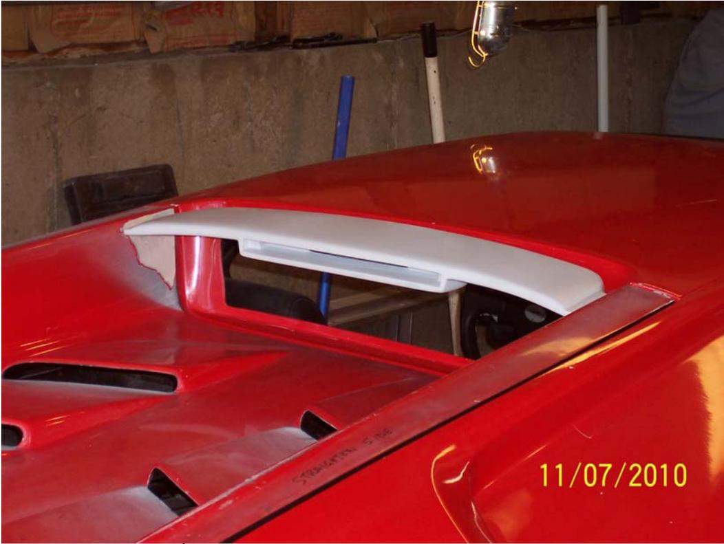
Designing 3<sup>rd</sup> light mount for engine hatch
