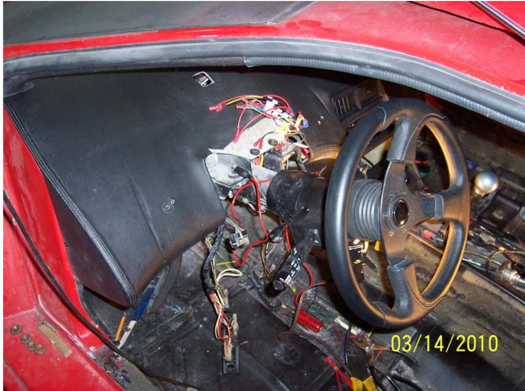
Wires for dash before gauge console is installed.
