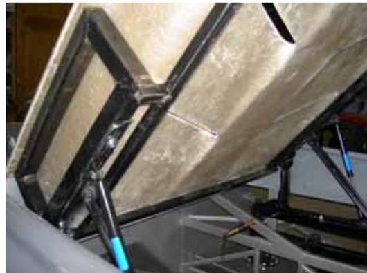
Viewing the engine deck lid mounted on the 4 brackets both hinges, you can see the installation works quite nicely. The Camaro hinges allow the deck lid to move back and up simultaneously.
