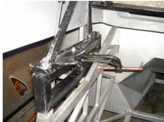
With this close-up view, you can see how the bottom hinge bracket sits on the tubular frame.
