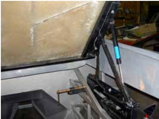
Looking at the passenger side, note the "C-clamp" used to secure the bracket for alignment. The deck lid should be raised and lowered numerous times before deciding it is in the right position.
