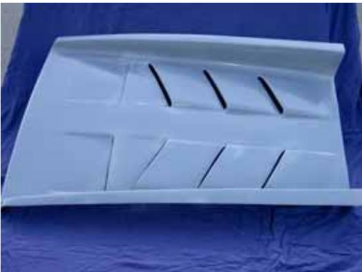
One problem with the hatch is its tendency for the front corners to curl in slightly. This requires a tubular frame to be manufactured for support and mounting of the deck lid.
