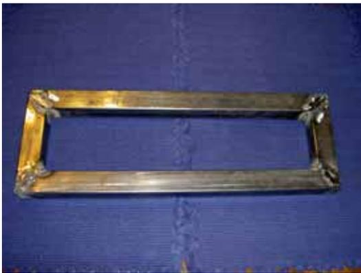
With the 1 1/4" square stock tubing, cut with 45 degree corner cuts (4) pieces 18" long (top and bottom of support/hinge frame), (2) pieces 6 1/2" long on outside (front uprights), and (2) pieces 6" long on outside (rear uprights). Layout the 4 pieces for each hinge frame and weld.
