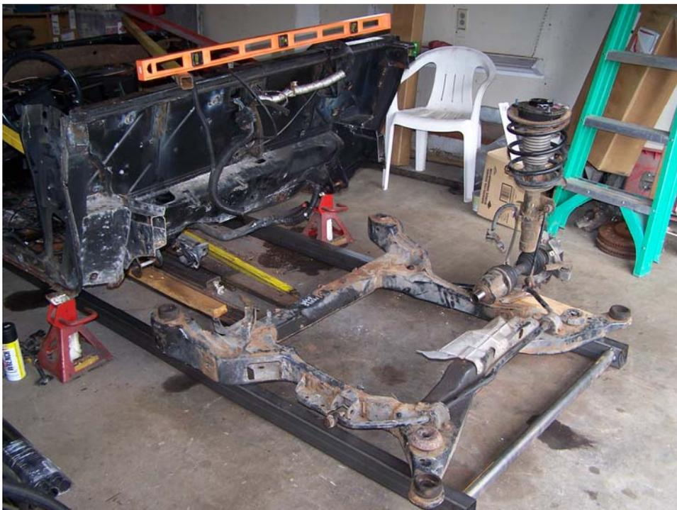
Pic #12 Cadillac Northstar cradle placed on jig to estimate space behind the firewall for fuel tank.
