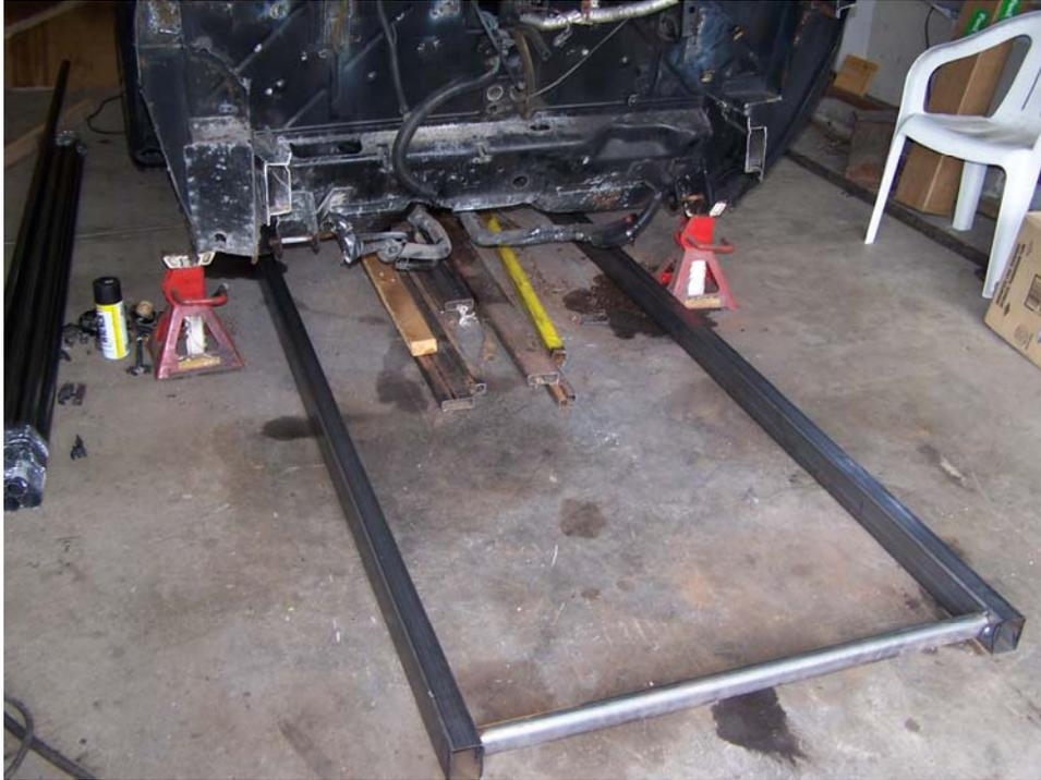
Pic #11 I made up a jig out of 2 x 3 tubing to keep things in alignment and straight. Once I get it level, it will be anchored to the floor.
