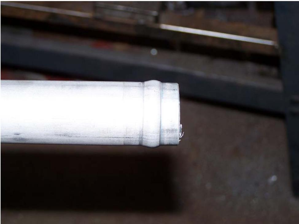
Pic 83 is an example of the tubing with the bead on it.
