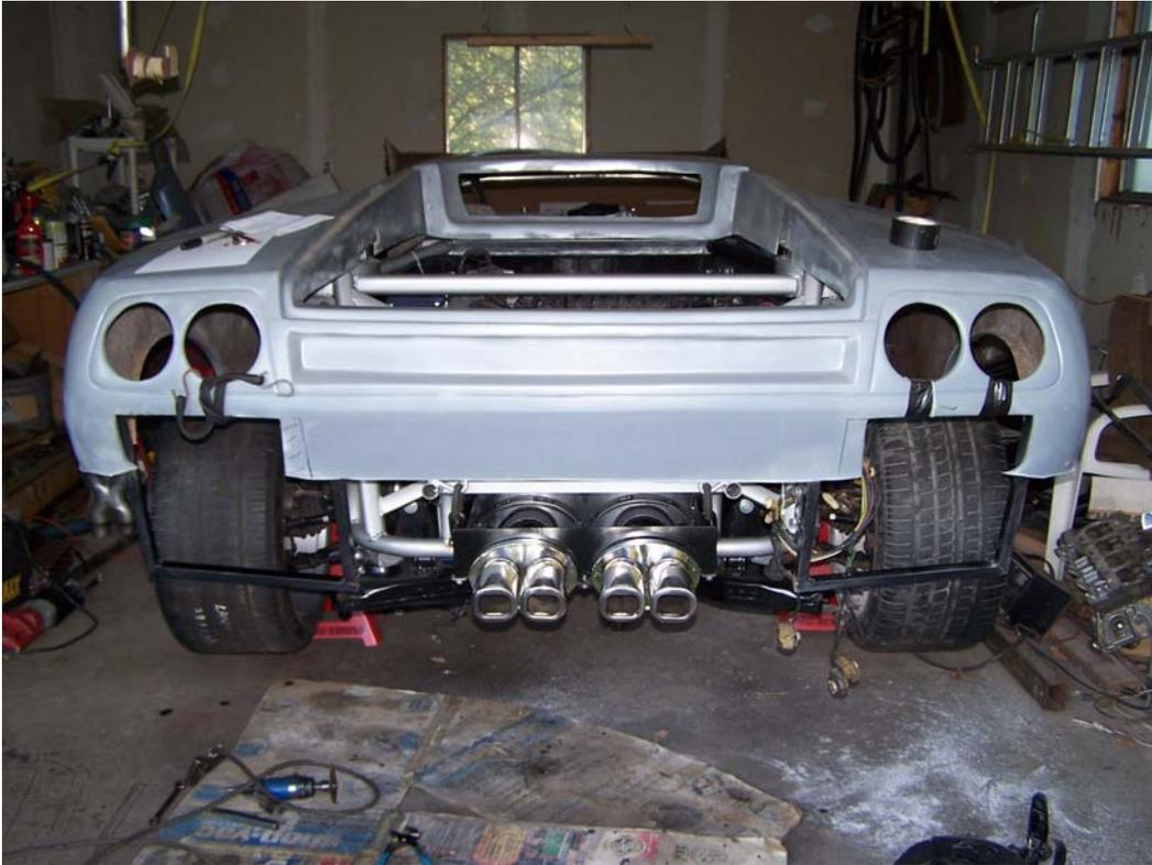
JC pic 78: Rear view of my Diabolic with mufflers installed. I cut the rear bumper off to redo the rear body. GTRs don't have a rear bumper.
