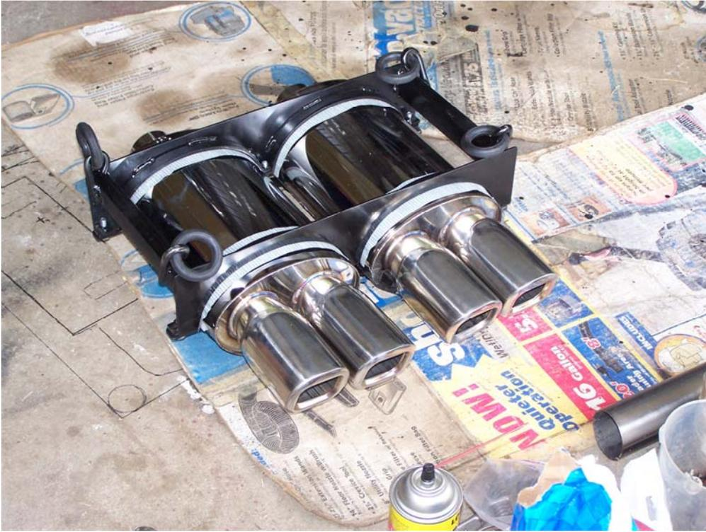
JC pic 76: Mufflers are temporary mounted in cradle for fitting.
