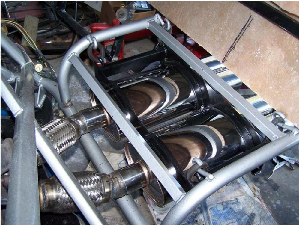
JC pic 77: Mufflers and cradle are mounted in chassis. I only ended up with 12" exhaust pipes.
