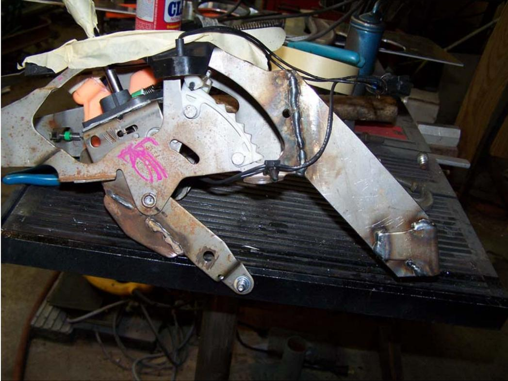
Pic 070 This is the cable retaining bracket welded on the rear of the shifter assembly.
