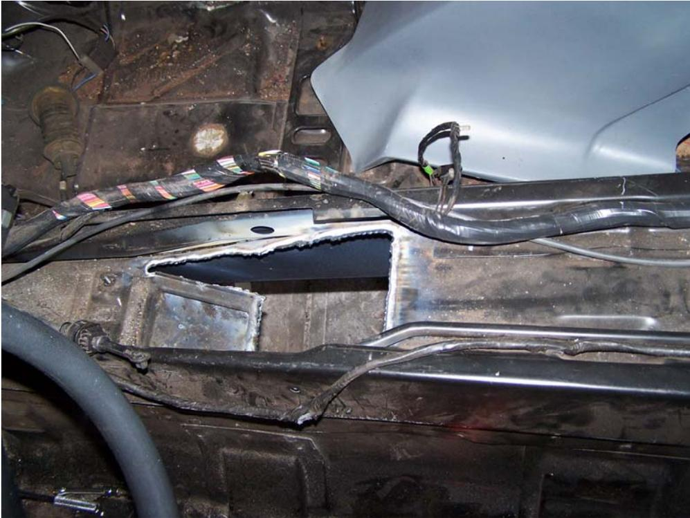
Pic 072 Here is the hole that I cut in the tunnel floor for the shifter with the rear cable. I am using a rear mounted fuel tank so there is plenty of area under the tunnel.
