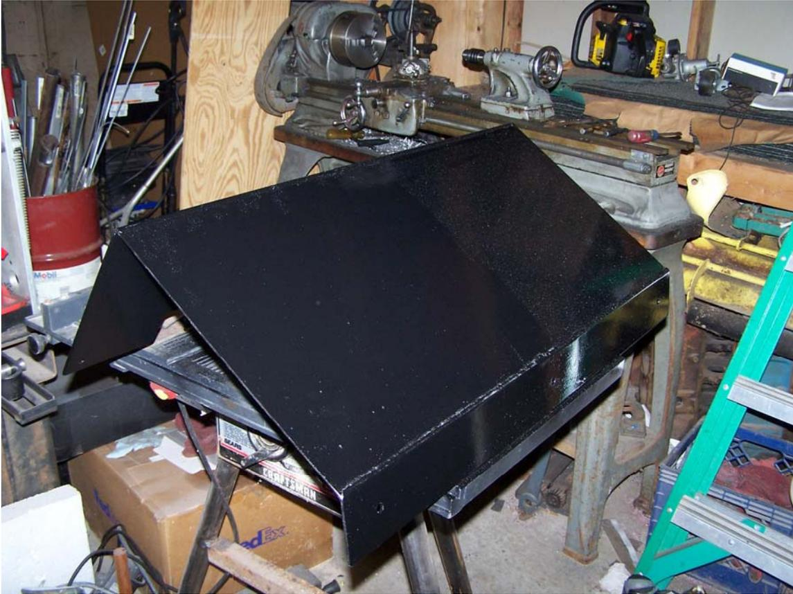
Pic 068 This is the Stone shield / Heat shield which I fabbed to fit around my fuel tank.
