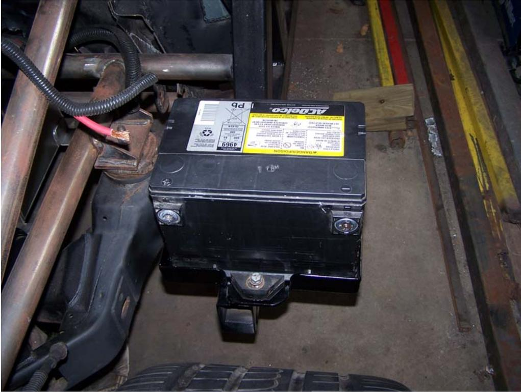
Picture 63 Shows the battery installed in front of the RH rear tire. Access will be through a panel in the wheel well housing.
