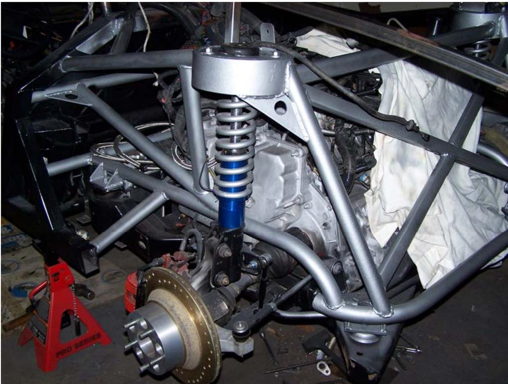
Picture 60 Shows a corner shot of the gusset at the rear strut top hat.
