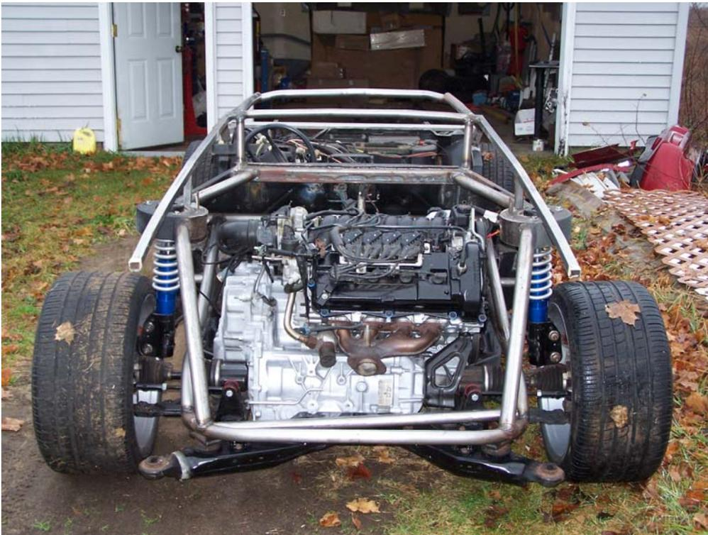
Pic #56 Rear View of chassis w/ Northstar installed with the 4T80 trans.
