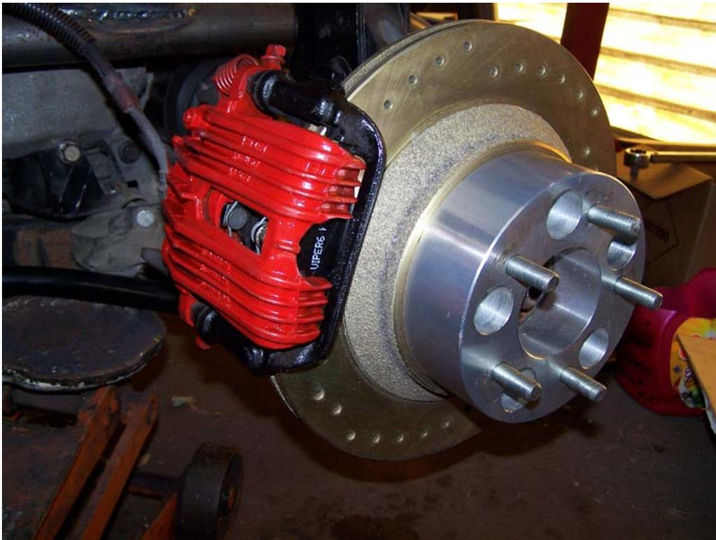
Pic #51. LH rear caliper mounted and looking good
