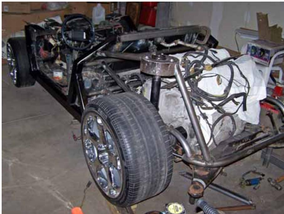
Pic #23. I have boxed the firewall with 2x3 rectangular tubing for strength and have welded strengthening tubes at the firewall cross tubing down to the lower cradle support tubing. The LH strut is now permanently welded to the firewall and to the lower tubing at the rear. More tubing will be added in the future to join the strut caps together as needed.
