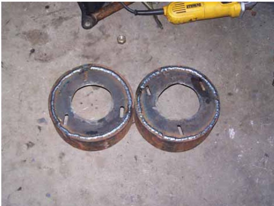
Pic #21. Here are my two strut caps ready to be positioned and welded in place. They were made from 8" diameter tubing with  $\frac{1}{4}$ " wall thickness.
