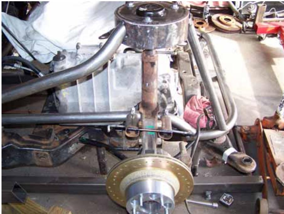
Pic #22. This pic shows my little strut alignment jig to hold the strut vertical. It was attached to the tube frame with two muffer clamps and was adjustable and worked well. The cap has been tack welded in the correct position before final welding.
