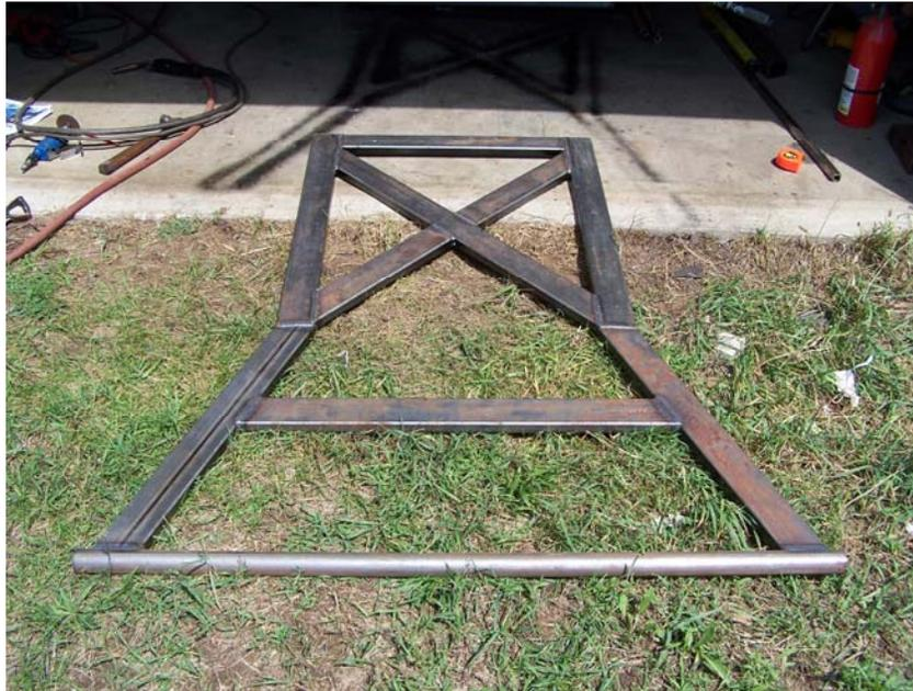
Pic #13 Slightly modified X-brace for Body strengthening after rocker reinforcements are welded in.
