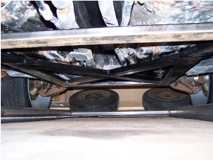
Pic #16 X-brace partially installed
