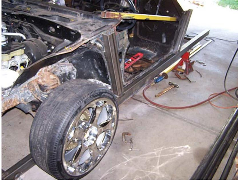
Pic #17 Body has been centered on floor jig and welded solid utilizing the rear cradle mounts on the firewall. Cadillac cradle has been centered and aligned to the rear wheel centerline. It is spaced 5½" ground clearance. Now comes the fun of building the tube framework.
