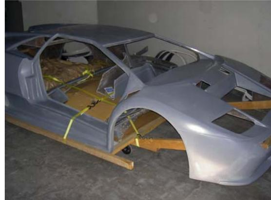
Note the side bumper rails (2" X 3" board) that extend 1 1/2" past body and keeps the body from hitting sides of freight vehicle. Tie-downs secured for the trip.
