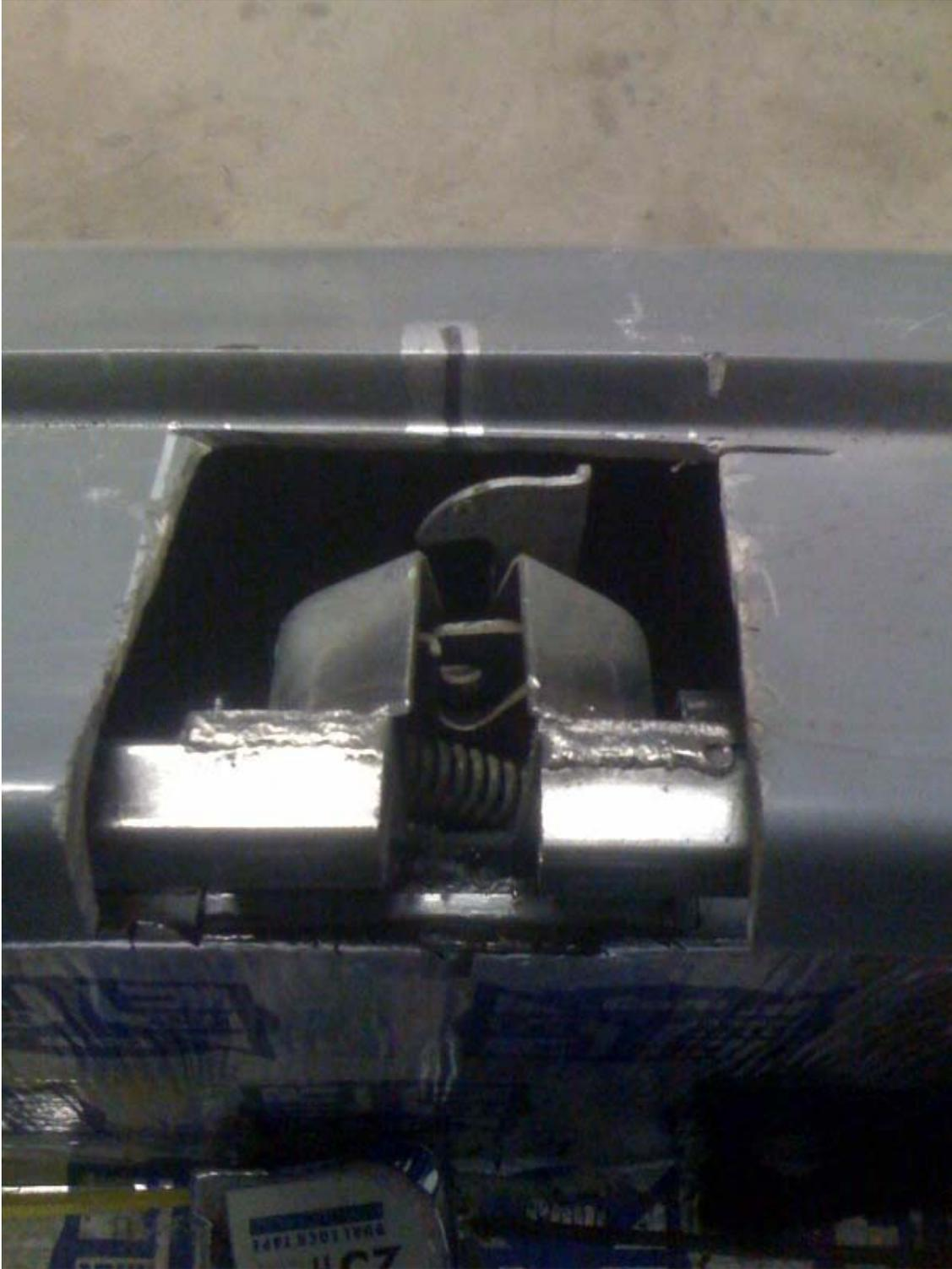
Hood latch is installed in cutaway area.
