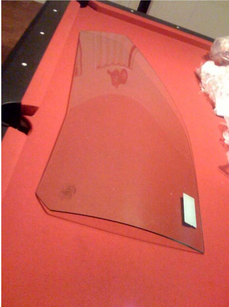
I really like the glass...looks really good. And I also like the bottom edges and the cut they made near the rear bottom of glass. That cut is so that when the window is all the way down, it doesn't hit the inner door. I won't be able to test fit until Sunday. I will send you follow up pictures soon!
