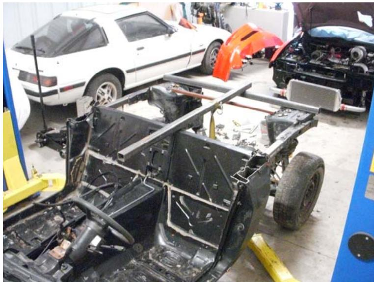
Once the unwanted chassis is cut away, Fellipe starts to weld on the modifications.
