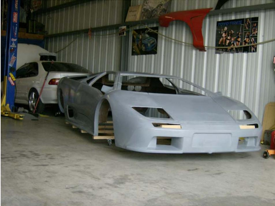
The wait is too long. The shipping pallet is removed and the body is being fitted to the modified Fiero chassis within 5 days of receiving the kit.
