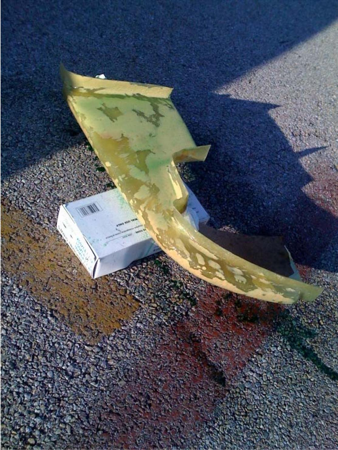
Prototype part made to cast mold off of
