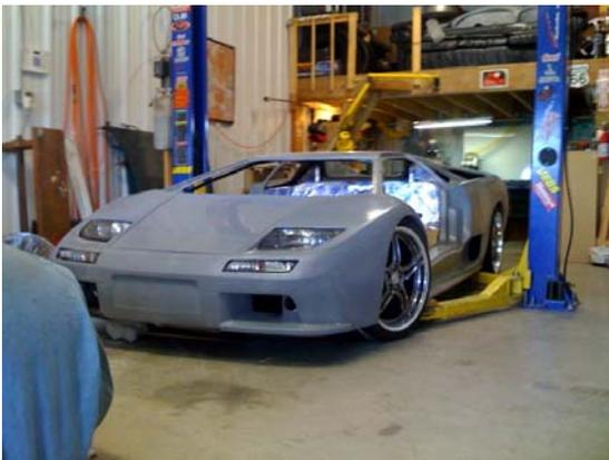
I still need to finish up the body work. But here is a rough look at the finish product. As you can see I'm still working on the carbon fiber lower pieces. I'm making a mold next week to fabricate better looking pieces.
