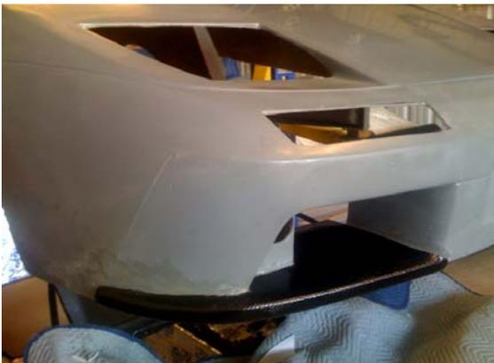
Black fiberglass with resin installed.
