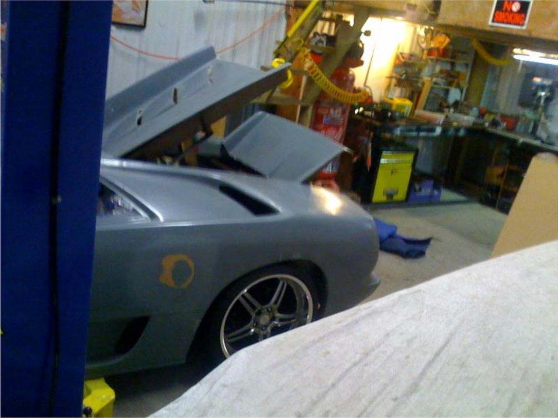
Split engine hatch modification and 20” rims and tires installed. Felipe is truly a **“Master of Automotive”**
