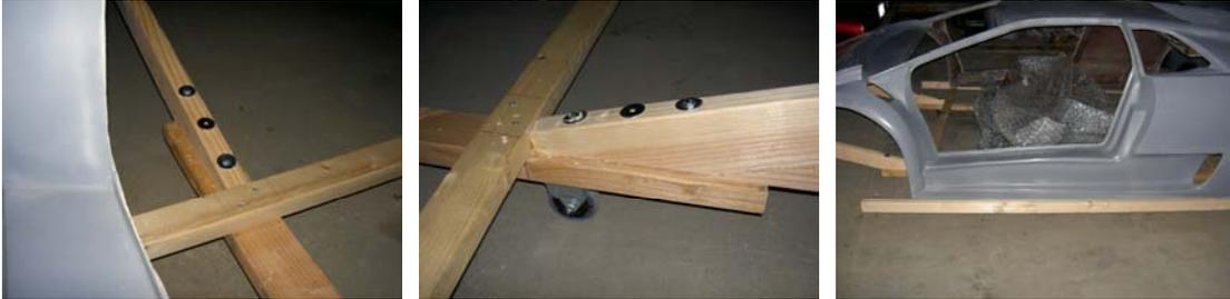
There are now a total of (4) of the 2” X 3” X 77” boards going across. Front and rear support struts are added with 3 lag bolts on each strut to secure each. There is also a “protective bumper board” added on each side of the body.
