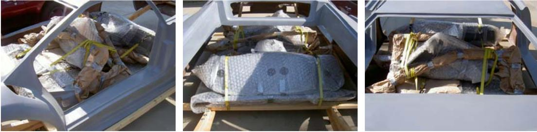
The paper and bubble wrapped parts are secured inside of the body to the body pallet with ratchet tie downs.
