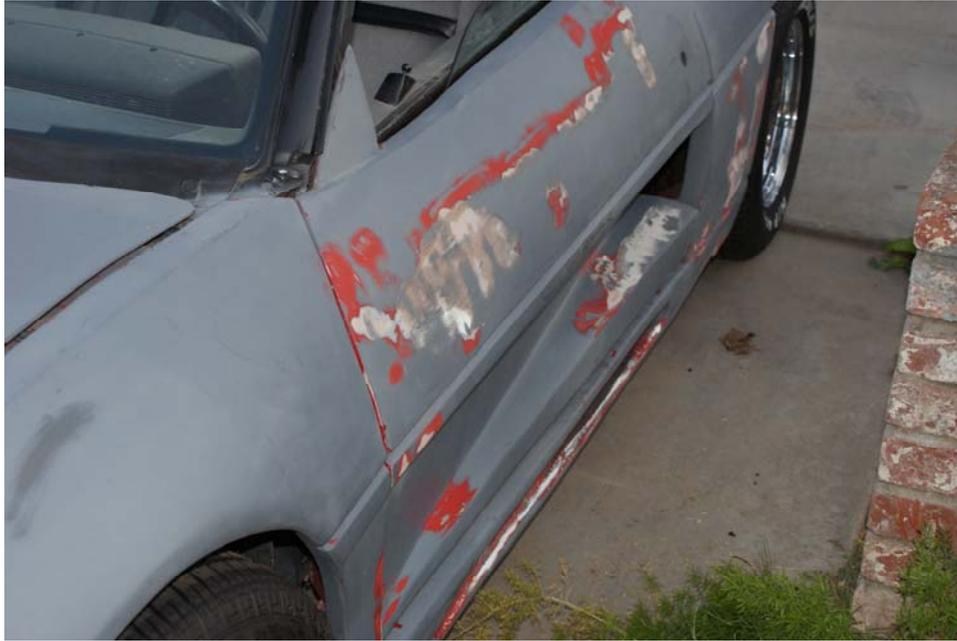
Picking up a used kit from someone that has started the project ALWAYS involves undoing some of the changes they have done. There is the cleanup of the fiberglass and repairs to the “hidden” damage they may have had.
