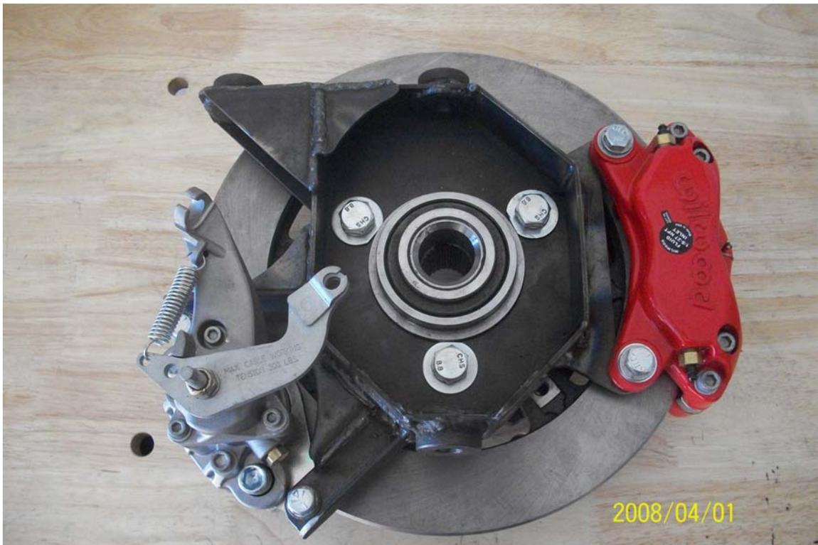
Disk brake assembly on spindle plate
