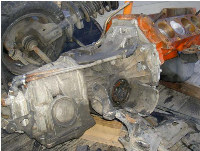
Axels removed from the Audi transaxle. Bolts require a metric “tri-square” tool.
