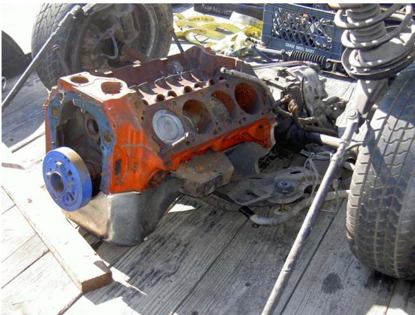
Dummy 351C block for measuring of motor mounts and transmission mounts
