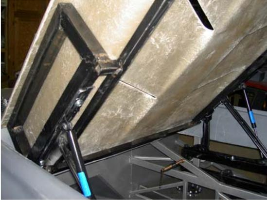
Fabricating engine hatch mounting
