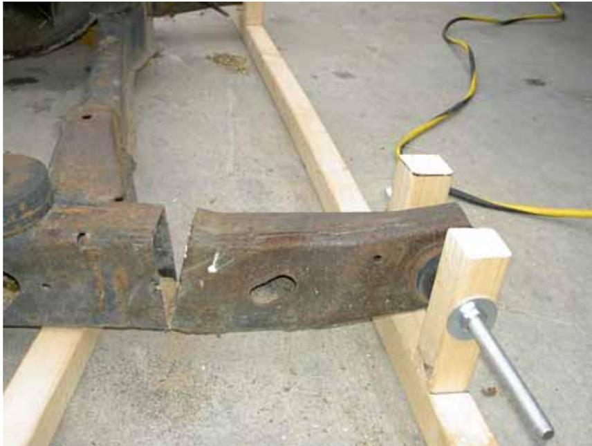
Both sides should be dropping equally, coming to rest back on the cradle jig. Complete cutting entirely thru the metal on both sides.
