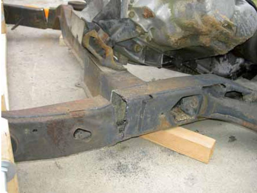
With both sides nearly sawed thru, the swing assemblies mounted on the jig will begin to fall and the frame will start to separate.
