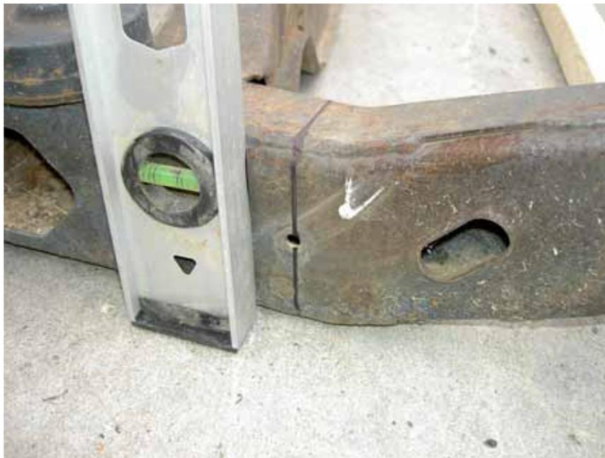
This is the vertical mark on the outside (passenger side). Note the hole (rivet removed) used as a reference point.
