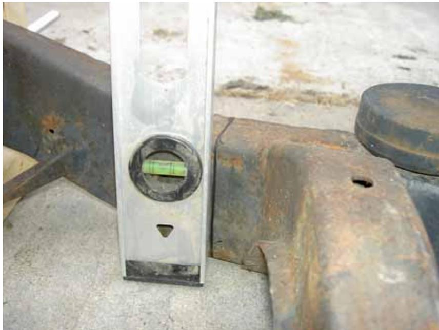
Now, using a level, draw a vertical line on the inside of each cradle tube. (Passenger side shown here – note narrower cross-member with more clearance to cut line)
