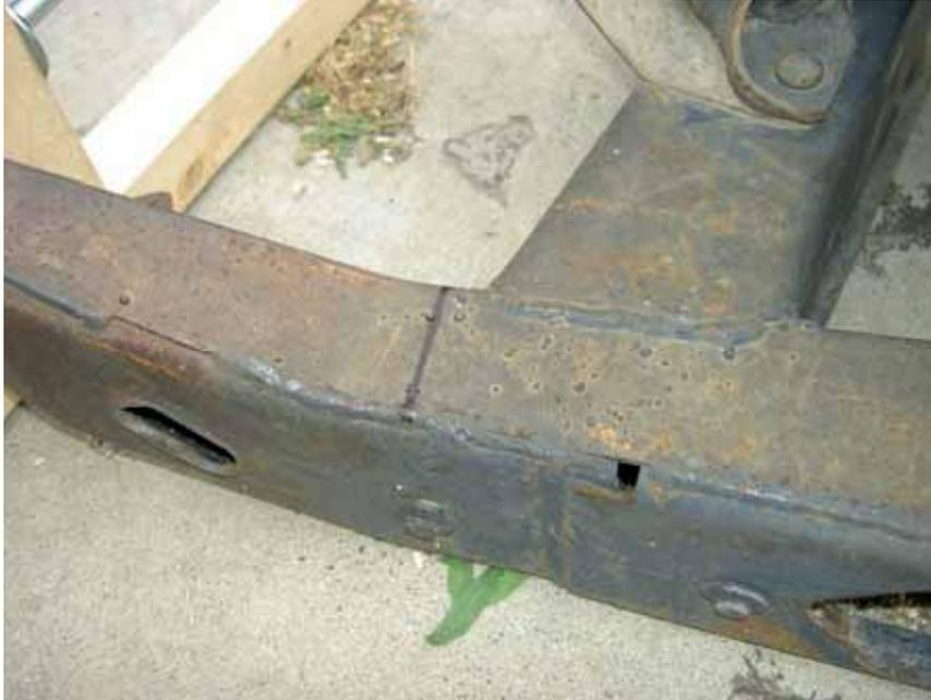
This line on the drivers side (shown here) will be close to the cross member, since the cross-member is wider on this side than the passenger side. (notice the hole and retainer rivet below the mark).
