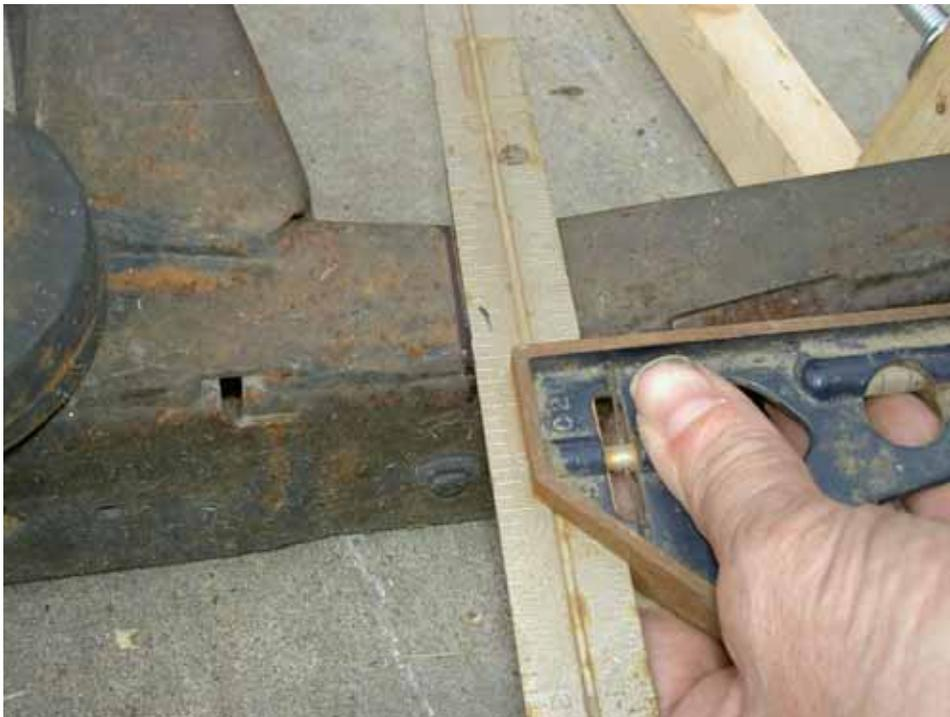
Use the same procedure on the passenger side. You can draw a line up thru the reference hole, and using the square to mark across the top of the cradle frame.
