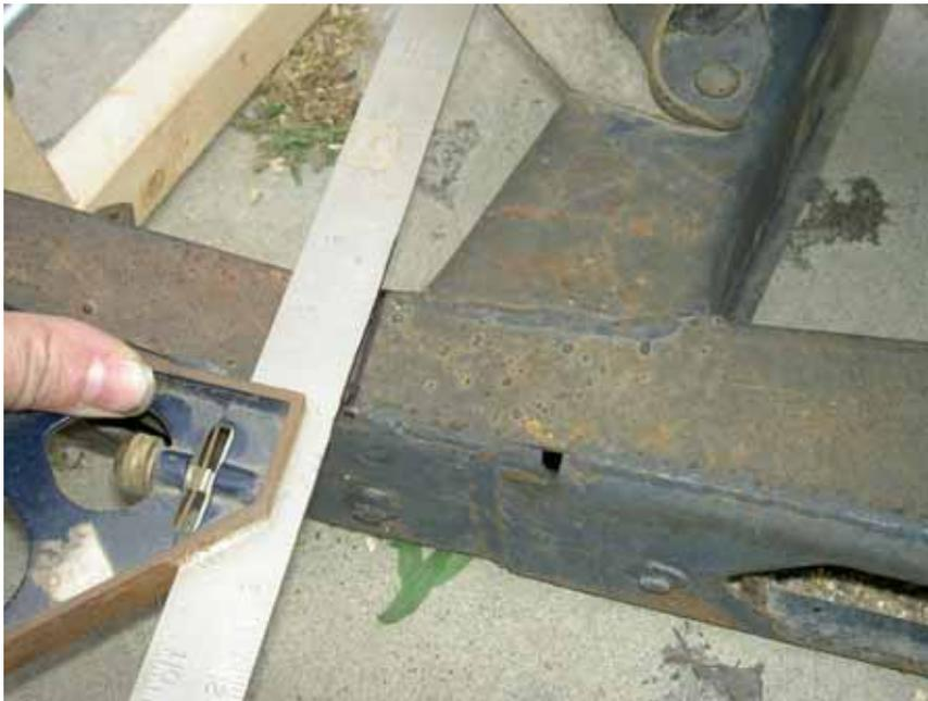
With a square on the outer surface towards the cradle pivot/mounting points, draw a line on the cradle square tube (drivers side shown here).
