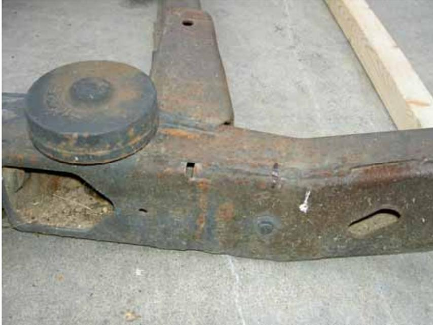
A mark is put at the 8" measurement, but actually could simply be drawn thru the holes on the outer side of the cradle.
