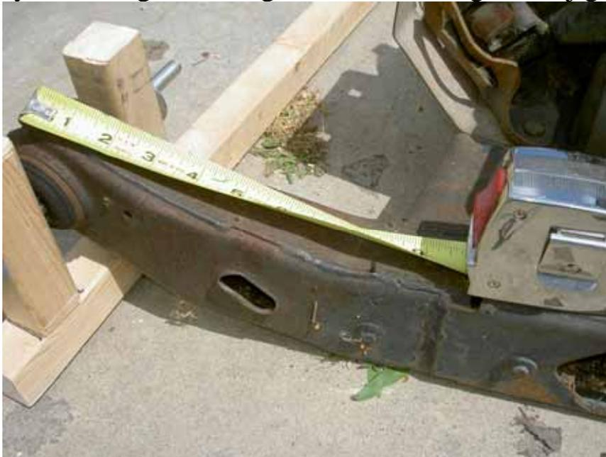
Measure 8" from the center of the pivot bolt. There will be a hole or retainer pin on the outside surface.
