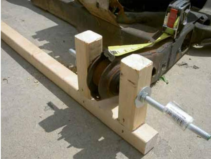
Note the cradle alignment jig that was made to keep the proper spacing of the cradle swing mounting points.
