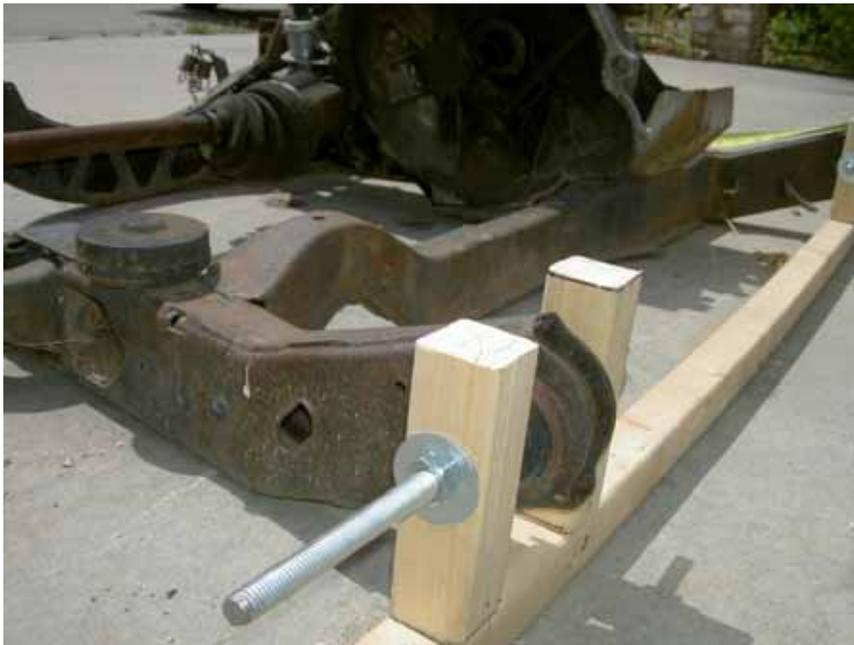
The jig can be manufactured out of wood or metal and will keep the pivot points the proper space above the ground level and will keep the two pivot points the proper distance between each other for future remounting.
