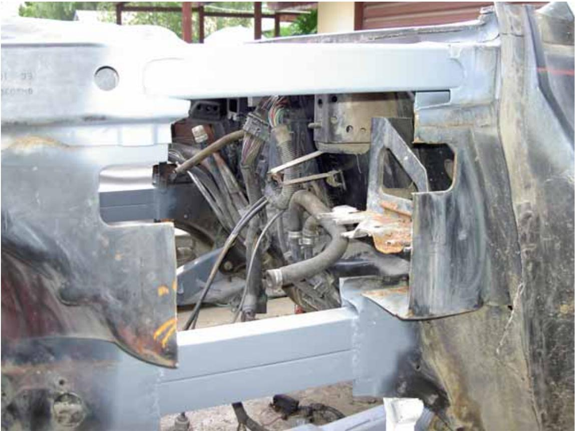
Extension tubes welded in on passenger side. Note that sheet metal can be added back in to cover the 10 1/2" opening created by the extension.
