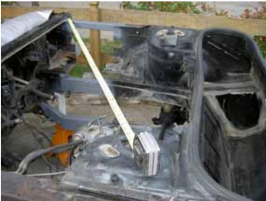
Once you have exactly 10 ½" (3" for F355, 7" for Countach) in between the front and rear frame cuts check for level again. Measure from the strut tower center hole diagonally over to the firewall opposite outer corner. The cradle frame should be able to be bolted back to the upper frame at the rear mounting points. This will help secure the alignment.
