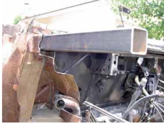
Making sure the chassis is level. Making sure the cradle is level. Making sure the upper extension tubes are level. Now the rear portion of the vehicle may be moved up and aligned to the extension tubes. The lower tubes will have to be pounded into the frame rails.
