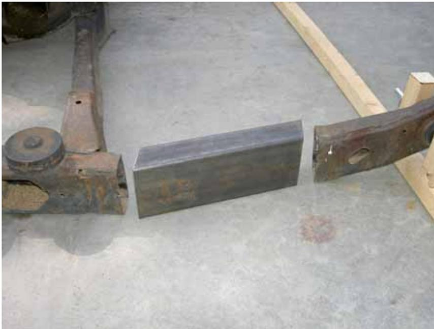
This is the other stretch tube for the cradle shown on the passenger side. Note both are identical but flopped over on opposite sides.
