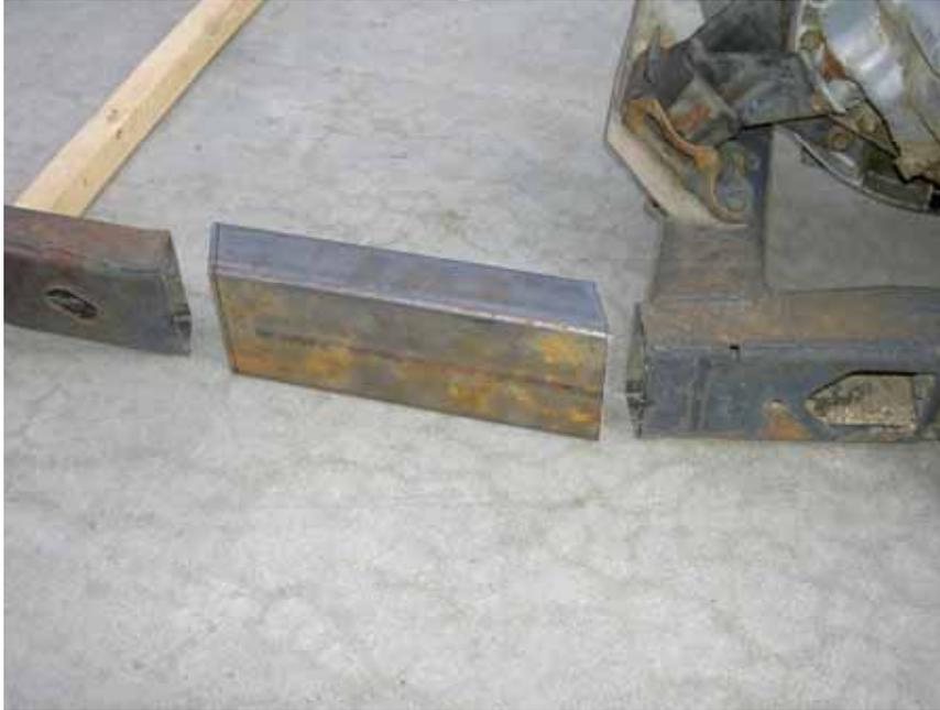
This is the stretch tube for the cradle (2 required) shown here on the driver side. These are available from B and B Customs.
