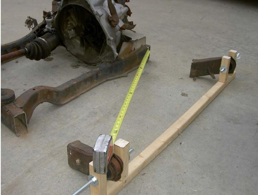
Now do the same but measuring from the drivers inside of the cradle to the center of the mounting bolt on the passenger side. This distance should be the same as the previous measurement (again  $39 \frac{1}{4}$ " in our case). Check this measurement both ways 3 or 4 times and move it slightly if not identical until both match perfectly. Remember to keep the space between the cut surfaces at  $10 \frac{1}{2}$ ".
