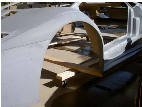
Body pallet is constructed with casters and mounted to body.
