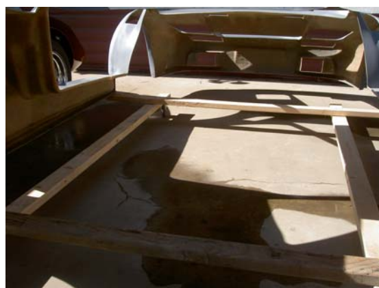
Body pallet is constructed with casters and mounted to body.
