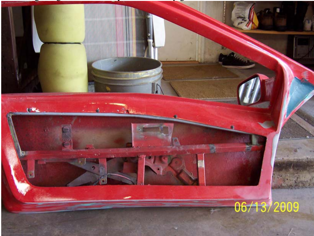
Reed H. getting the doors ready to have rollup glass installed
