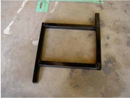
This is the tubes welded up before the mounting tabs are welded on.
