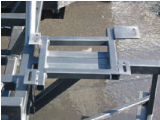
Two tubes are welded across the base (as illustrated) to allow the bracket to be slid in and out. The slots in the mounting tabs are slotted to allow the headlight to be adjusted forward and backward.
