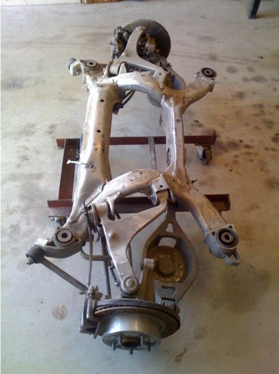
2006 Nissan 350z complete rear end assembly. All Aluminum too!!! Super light weight. It's got slotted/drilled rotors too! When I install it on my frame I will cut off the center section to give the new engine and transaxle room...then I will build 2 new lower support bars. I paid!
