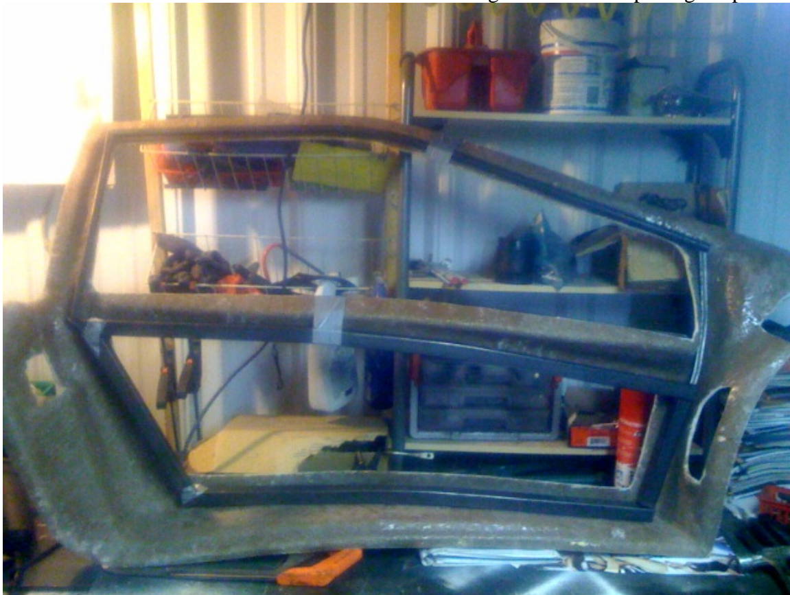
The frame is constructed for the doors and will be fibreglassed in to keep things in place
