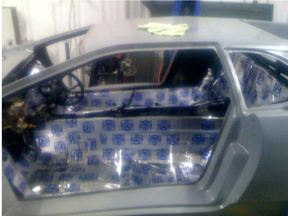
The frame is constructed for the doors and will be fibreglassed in to keep things in place
