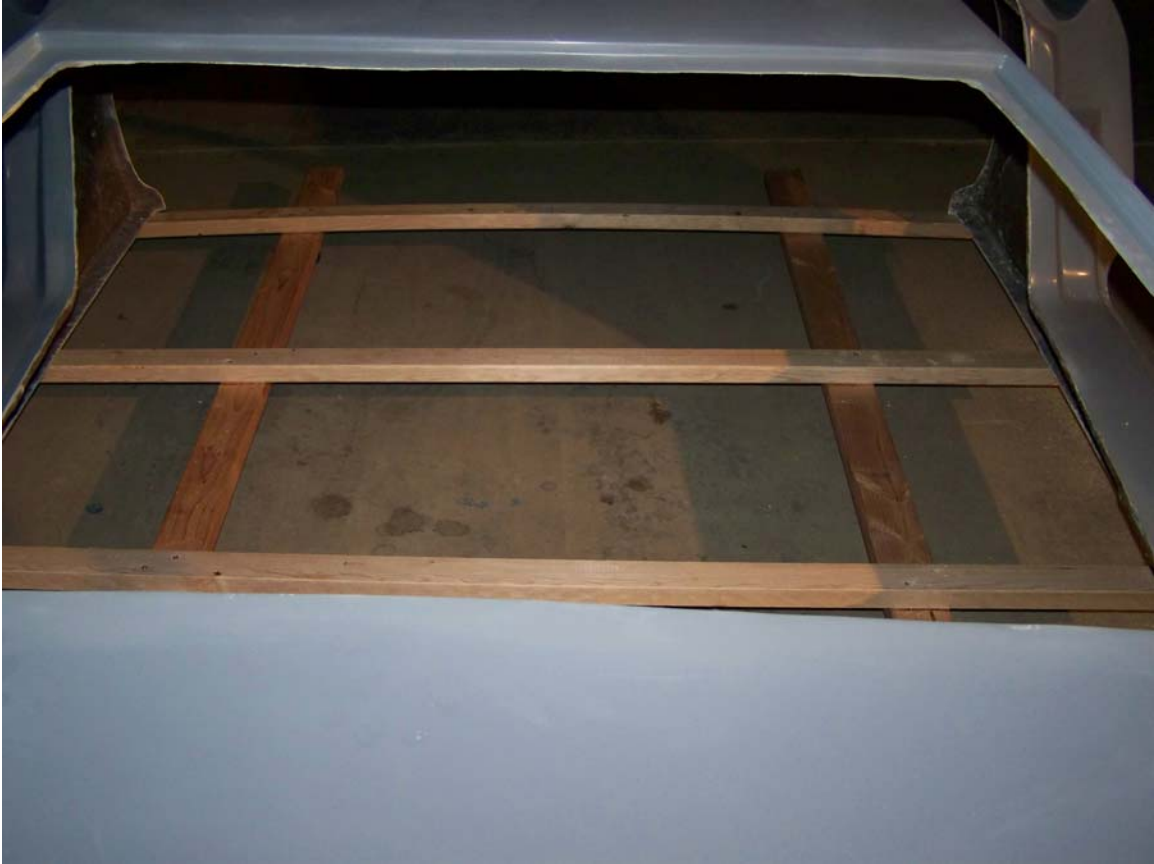
Looking through the front window at the runners and cross members. The end cross members are secured with wood screws through a fender washer and thru small mounting holes in the lip of the body shell.
