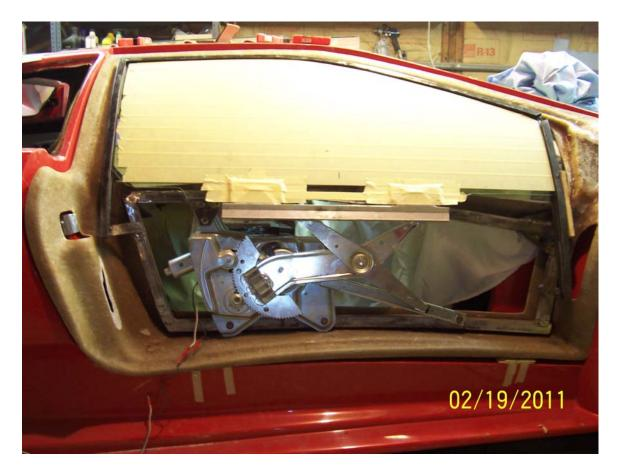
I'm using D&R glass. It is shorter so you don't have to cut the door frame. T-Bird window channels, and the regulators are from a 95-99 Monte Carlo
