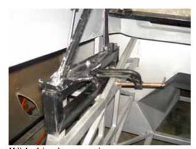
With this close-up view, you can see how the bottom hinge bracket sits on the tubular frame.
