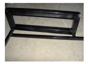
Note the  $2\frac{1}{2}$ " extension of the front lateral frame tube and the  $1\frac{1}{2}$ " rear hinge frame supports welded in place. The outer edge of these tubes are welded underneath and flush with the outside edge of the hinge frame.
