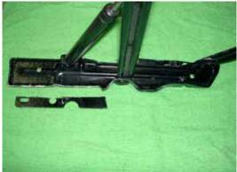
The sides of this section need to be trimmed off, leaving just the rounded corner to keep the strength and rigidity of the hinge. This is to allow clearance for the hinge and not drag on the body surface when the rear hatch rises.
