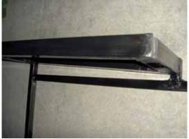
Looking from the top view, you and see the longitudinal frame tubes move outward from each other (29" apart in the front and 37" apart in the rear).
