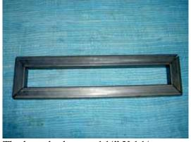
The lateral tubes are 1 <sup>1</sup>/<sub>4</sub>" X 1 <sup>1</sup>/<sub>4</sub>: square tube cut of at a 45 degree angle with 18" on the outside edge. The vertical tubes for the bottom hinge mount are 1 <sup>1</sup>/<sub>4</sub>" X 1 <sup>1</sup>/<sub>4</sub>" tubes 4 <sup>1</sup>/<sub>4</sub>" long on the outside of the 45 degree cuts. When the 4 tubes are welded together, they form a 4 <sup>1</sup>/<sub>4</sub>" by 18" boxed frame as shown in the above picture.
