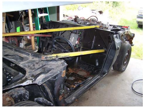
Pic #7 Passenger compartment braced for major cut behind firewall
