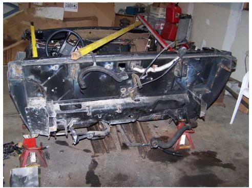
Pic #10 Rear firewall cleaned up after removal of gas tank.
