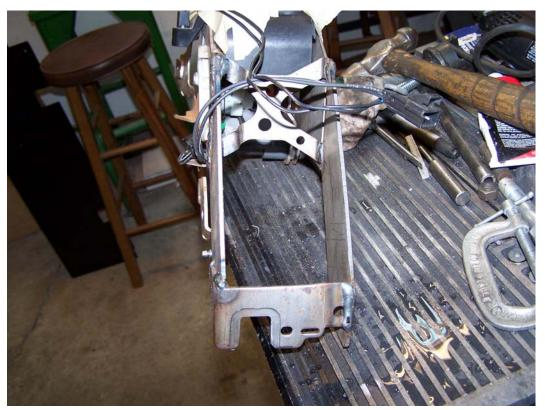
Pic 071 Another picture of the shift cable retainer slot in the rear mounted bracket.
