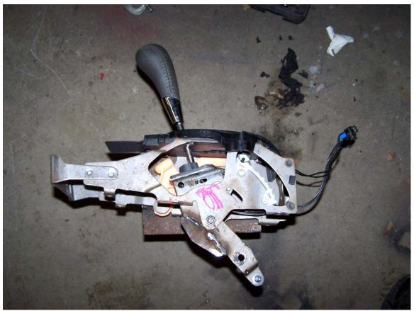
Pic 069 This is my Oldsmobile Aurora console shifter that had to be reworked to operate a shift cable mounted from the rear of the car.
