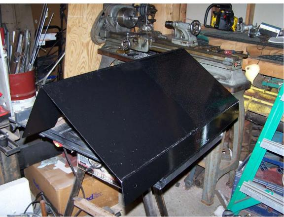
Pic 068 This is the Stone shield / Heat shield which I fabbed to fit around my fuel tank.
