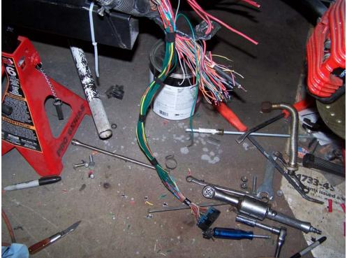
Pic 064 I had to lengthen one of the engine harnesses 21" to reach the fuse box. I don't remember reading that in the instructions???
