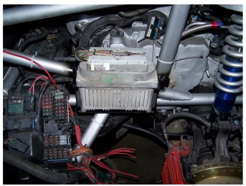
Pic 067 Fuse Box and CPU at home just in front of the LH rear wheel. I will fab an access door in the wheelhouse for access if needed.
