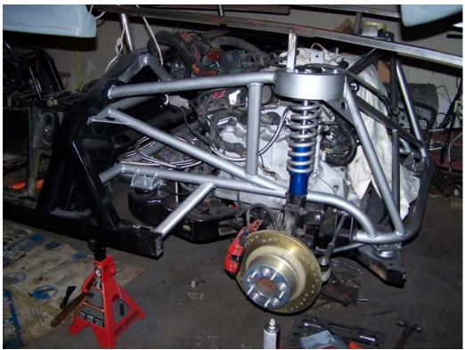
Picture 59 Shows the additional strut in front of the LH rear strut and the connector strut connecting the side rocker rectangular tubing to the rear round tubing.
