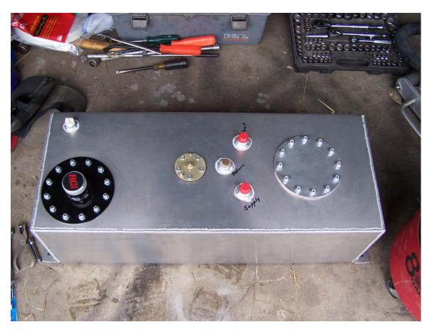
Here is a picture of my fuel cell. I had to relocate the filler neck and the fuel bypass fitting as they interfered with my structural tubing. Minor problem. All that remains with the fuel cell is the attachment framework and stone shield/heat shield and we should be ready for some fuel lines and fittings.
